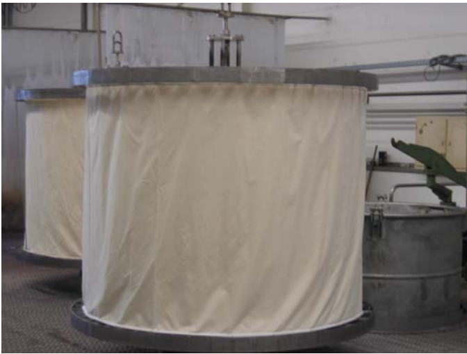
Star dyeing mcs. – single, double and triple vertical stars
