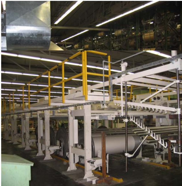
Beam creel - 9 positions installed , air break controlled
