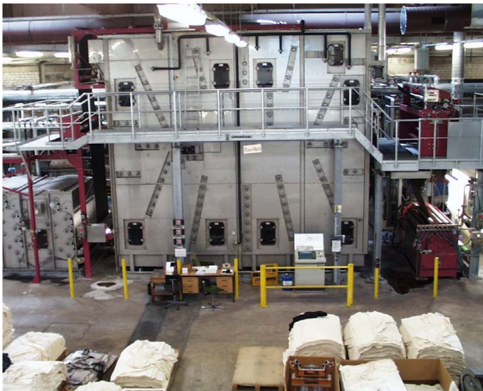
Spiral steamer – 120 m content , all rollers driven by independent fu controlled motors
