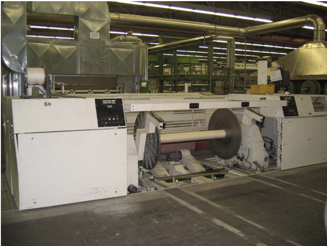
Sucker Mueller slasher – yoc 1997 , ww 2600 mm for beam diameters of 1250 mm
