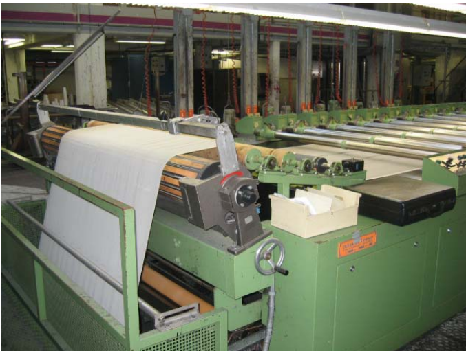
Zimmer Rotary printer – 9 colours
