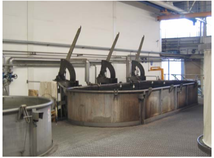
Star dyeing mcs. – single, double and triple vertical stars
